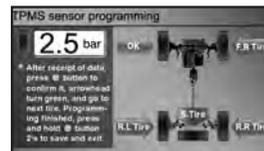
The system will receive the sensor signal and the corresponding tire pressure value will be showed on the monitor. Press the remote button once to confirm the programming.
