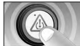
25 seconds after ACC on, press the remote button 5 times to enter the sensor programming interface
