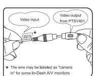
3. Insert the video output plug into the video input socket of the In-Dash A/V monitor.
