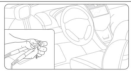
1. Identify the reversing light wire (+) in the driving compartment.
