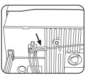
Connect the reversing light wire (+) with the reversing signal input wire at the back of the In-Dash A/V monitor.
