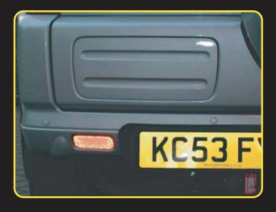
A-Sensor is mounted at approx 54cm from the ground.
