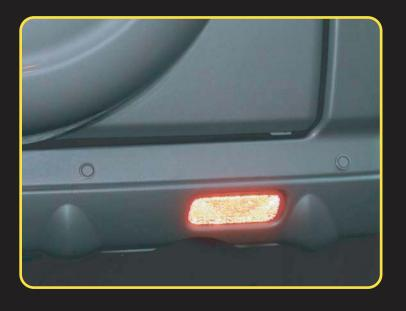
D-Sensor is mounted at approx 54 cm from the ground.
