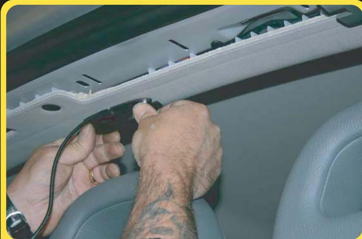
Remove the plastic trim situated at the rear of the headlining that covers the headlining retaining clips.
