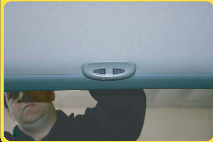
Make sure you are confident that the display is central and square then screw up to the headlining and clip on the display cover. There is no need to cut headlining to allow cable to go through as cable can run directly under rear headlining plastic trim.
