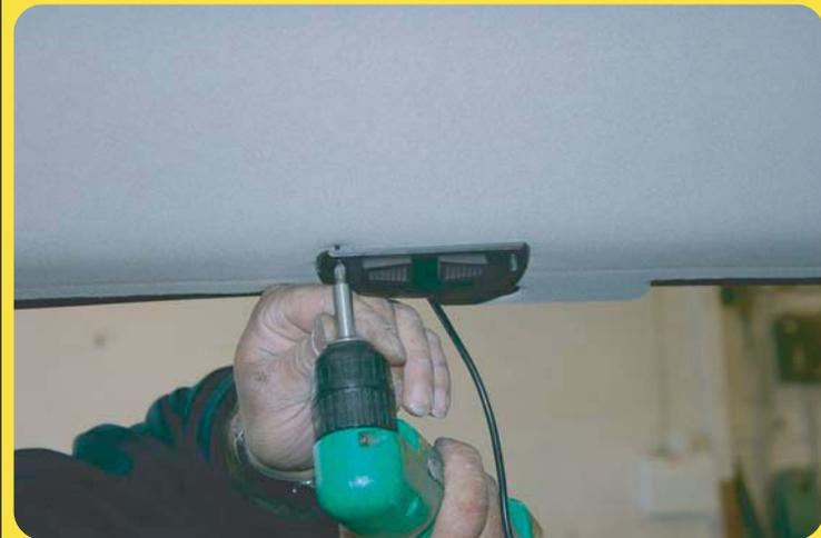
The centre of the vehicle is easy to find as there are two cutouts side by side in the metal part of roof at the rear, the left hand side cut out is the centre marker.
